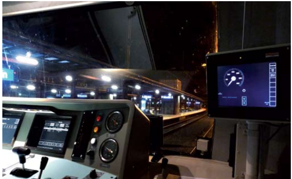
Cab view from a Class 471 EMU showing the AVV display (centre) and ETCS DMI (right).
