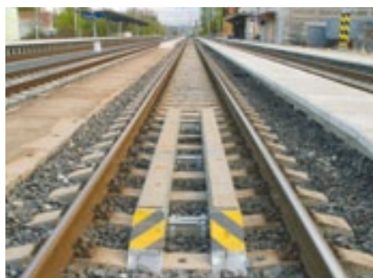
Information balise at the track
