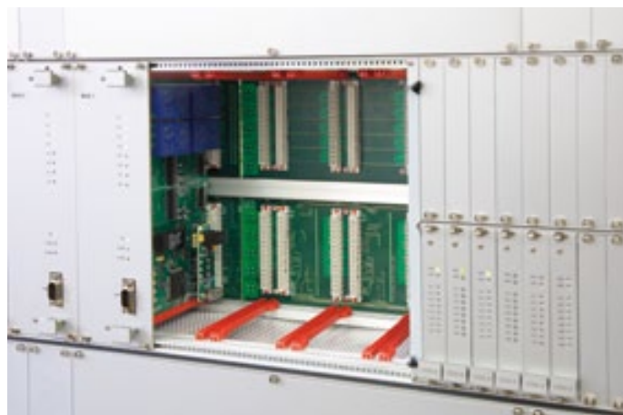
AVR3 Unit of the TCR track receiver set
