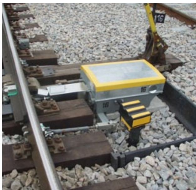
Fixation of machine by toggle mounting set
