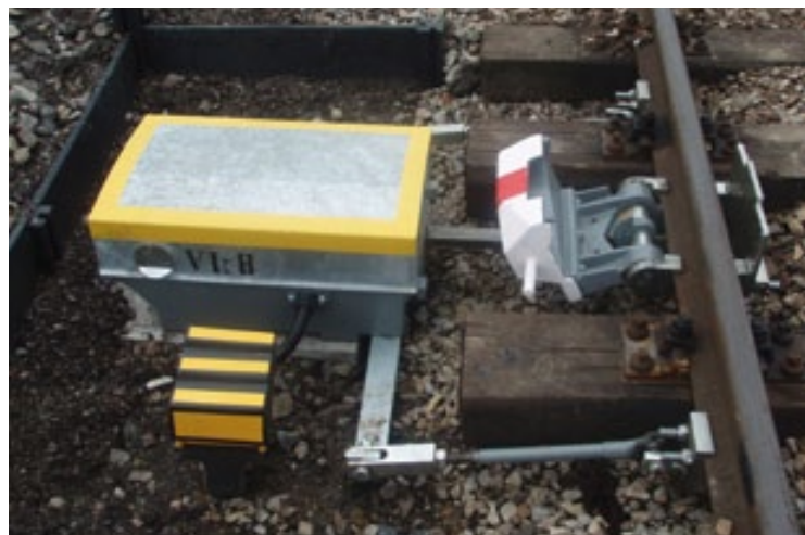
Derailer effective position
