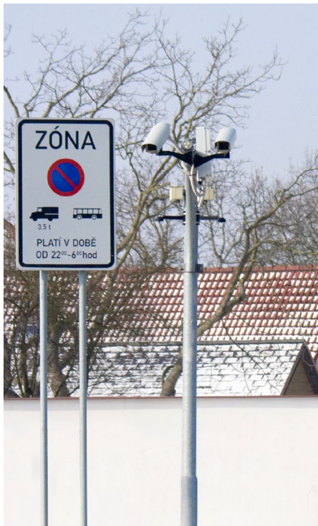
Stand with CCD cameras and infrared reflectors
